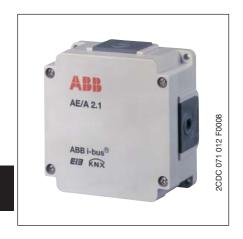
Analogue Input AE/A 2.1 is used to record analogue data. Two conventional sensors can be connected to AE/A 2.1. The connection to the bus is established using a pluggable screw terminal. The device is ready for operation after connecting the bus voltage. No additional auxiliary voltage is required. Analogue Input AE/A 1.2 is parameterised and programmed using the ETS
